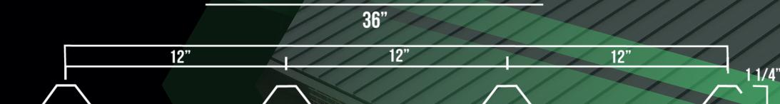
PBR Panel is what many would consider to be the standard for commercial and industrial uses. Because of its higher ribs and thicker gauges, PBR is what many would see on warehouses or larger buildings. Magnum carries this line in all of our popular colors and while the standard is 26 gauge it can also come in 24 gauge as well.
