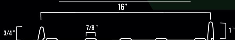
Standing Seam would be considered Magnum Metals "top of the line" panel for the roofing application. It is a residential and architectural panel. Many would see this on higher end homes and buildings. Because it is a locking panel system, all of the fasteners are hidden and boasts of a look like no other. Available in 26 and 24 gauges and many colors, this is what many would consider to be the only way to go on a roof for their home or business.
